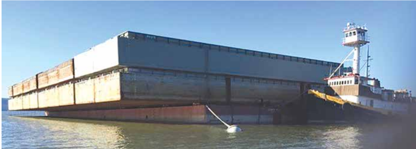
Barges on top of barges – a fleet of canal barges planned for use on the New York State Canal System makes its way north, courtesy of a seagoing tug. The barges are especially suited for the canals, being the right size, shape and draft to maximize the amount of cargo capacity on these narrow, relatively shallow waterways that limit maneuverability. Photo courtesy of Sea Tow.
