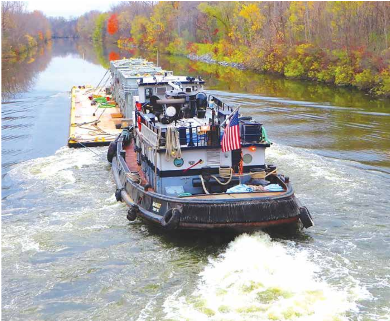
The tug "Margot", with pilot house lowered to clear low bridges in western NY, pushing a cargo of generators on the Erie Canal. A modern variation on "low bridge, everybody down", the "Margot's" telescoping pilot house enables it to politely duck under bridges and move its cargo to the most remote locations in New York State and beyond. Photo courtesy of Bob Stopper, Lyons
