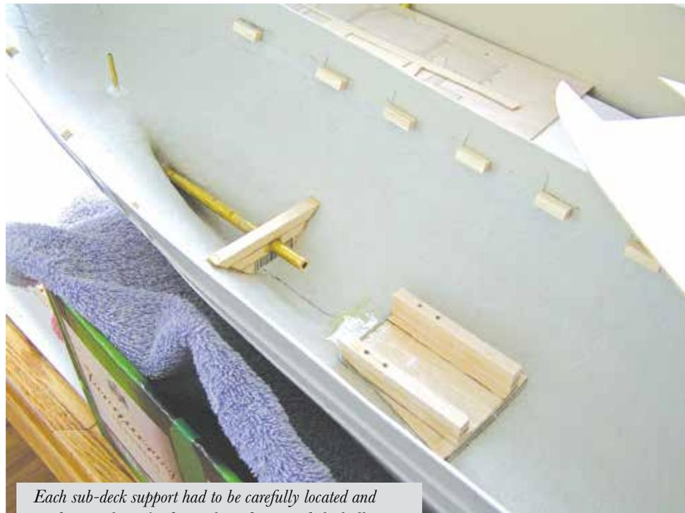
*Each sub-deck support had to be carefully located and conform to the entire forward to aft curve of the hull. Measured from the top edge of the hull after it was faired. 6 Minute, 2 part epoxy was used.*
