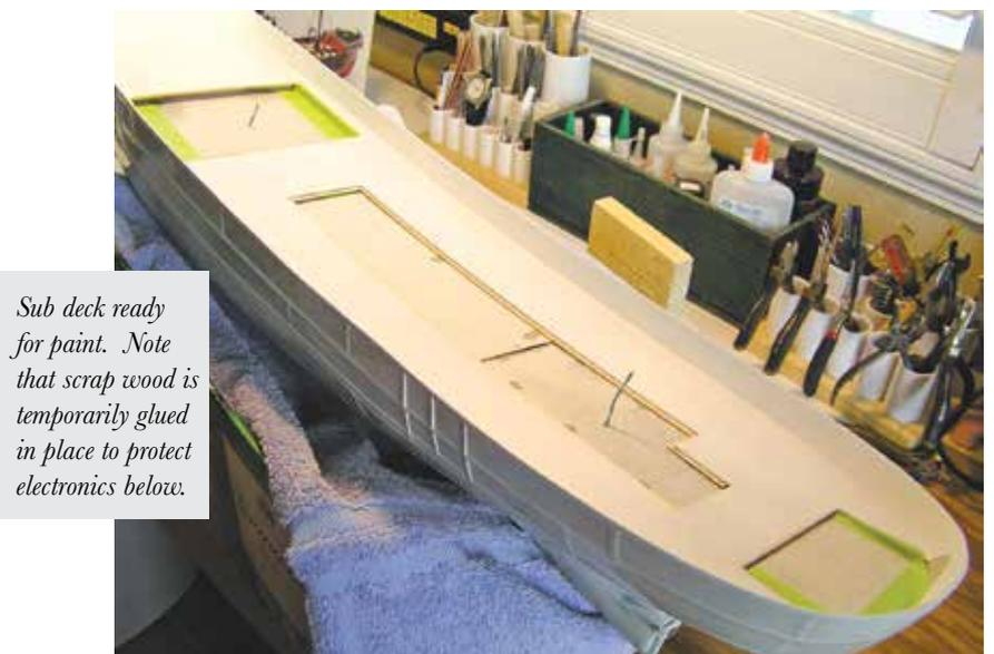
*Sub deck ready for paint. Note that scrap wood is temporarily glued in place to protect electronics below.*
