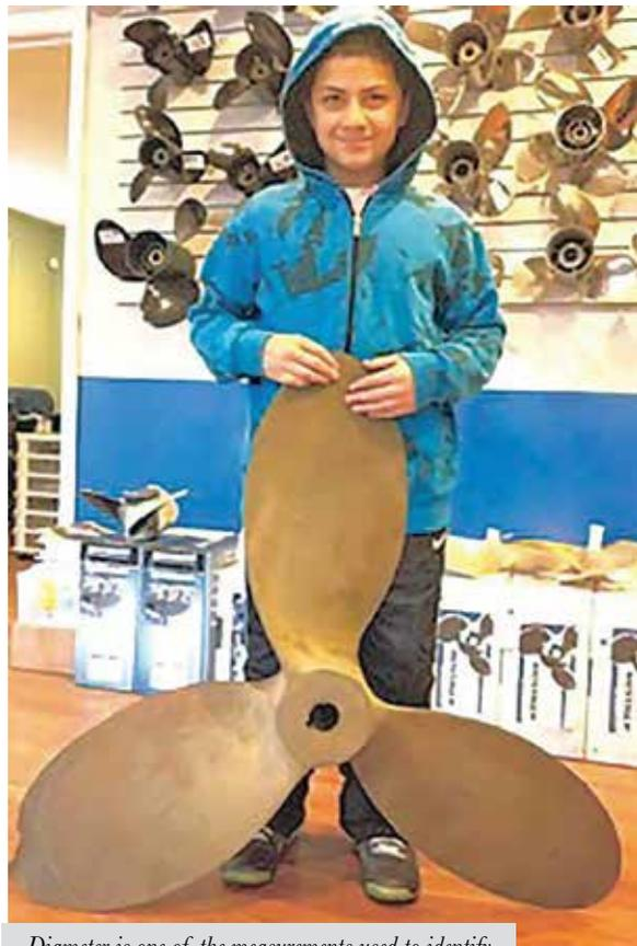
Diameter is one of the measurements used to identify a specific prop. The diameter of this propeller is 42 inches, as illustrated by my nephew.
