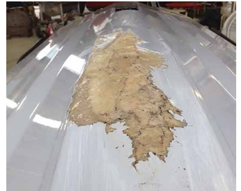
Note darker area along left side of damage is wet out with resin better than lighter area. Very dark area indicates holes in the laminate
