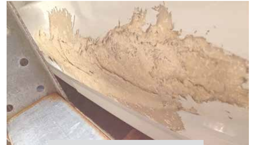
Note darker area along left side of damage is wet out with resin better than lighter area. Very dark area indicates holes in the laminate
