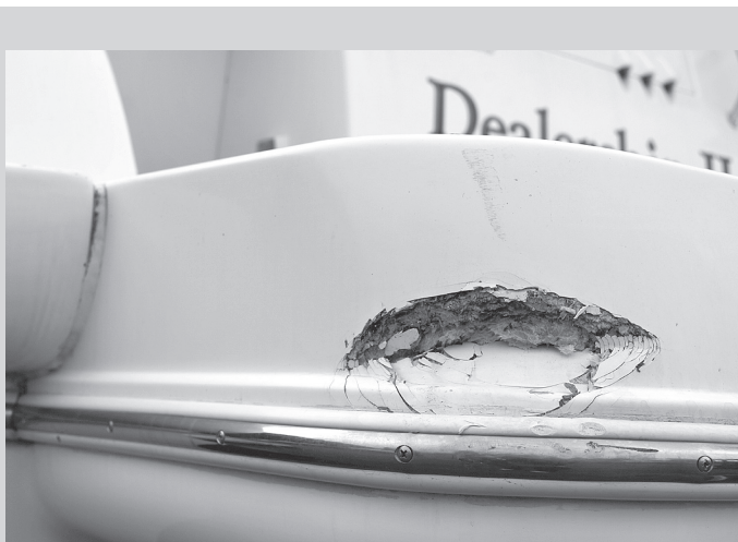
The Cruisers boat featured in May 2012 Issue is nearing completion. See cover photo. Images shown are of the repair in progress on the big hole caused by a 10" cleat being torn out of the starboard side transom.
