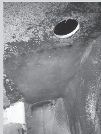
The Cruisers boat featured in May 2012 Issue is nearing completion. See cover photo. Images shown are of the repair in progress on the big hole caused by a 10" cleat being torn out of the starboard side transom.
