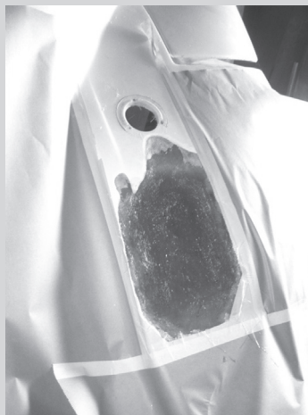
The Cruisers boat featured in May 2012 Issue is nearing completion. See cover photo. Images shown are of the repair in progress on the big hole caused by a 10" cleat being torn out of the starboard side transom.
