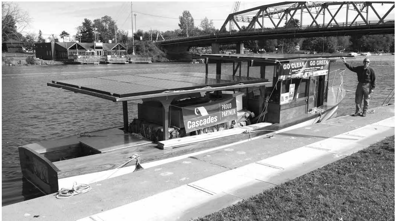
Professor David Borton stands beside the Solar Sal hull prototype that completed the historic 2015 trip. Viewed at the docks at Brewerton, NY in October 2015, Solar Sal is carrying an 8000 lb payload, or the equivalent of 30 passengers plus gear. The trip was made exclusively under solar-electric power. Photo courtesy of the Chamber of Southern Saratoga County
