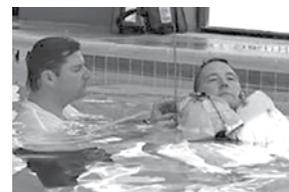
relative to that of the DeckVest. The Winner has a crotch strap that proved beneficial in keeping the jacket from riding up. The Winner relies on a zipper that separates upon inflation, and in theory, makes the unit easier to repack. However, testers discovered that the zipper sometimes came apart when it wasn't supposed to.
